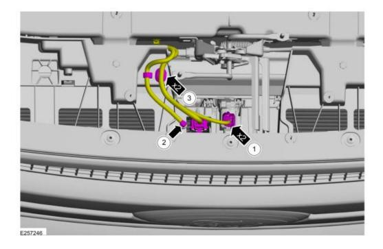
1.3 On both sides, remove the 2 screws. *Torque*: 15 lb.in (1.7 Nm)
