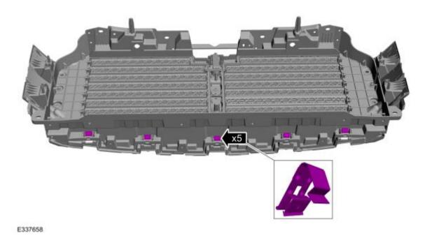
1.11 Remove the screw and the nuts. *Torque*: 1: 22 lb.in (2.5 Nm) 2: 44 lb.in (5 Nm)
