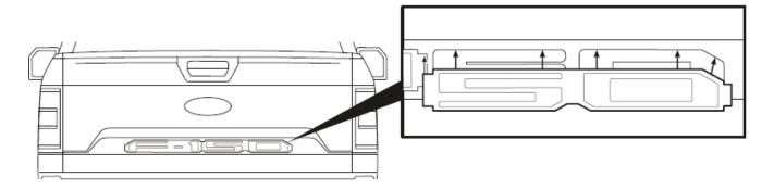
2.5 Use the foam block to firmly press along the directions shown in the illustration below to adhere the decal to the tailgate.
