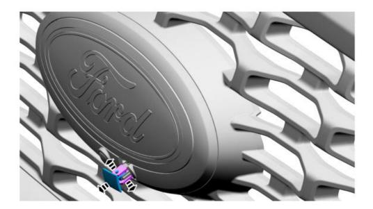
1.18 Remove the screws and the front camera washer and bracket as an assembly.
