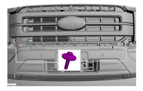
1.7 Remove the pin-type retainer. Pull up to disengage the locating pins along the top of the grille. Pull forward on center of the grille to remove.
