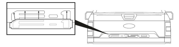
2.3 Use the foam block to firmly press along the directions shown in the illustration below to adhere the decal to the tailgate.
