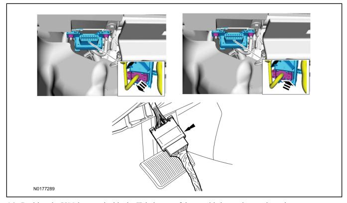
16. Position the VSS harness inside the IP being careful to avoid sharp edges and moving parts.
