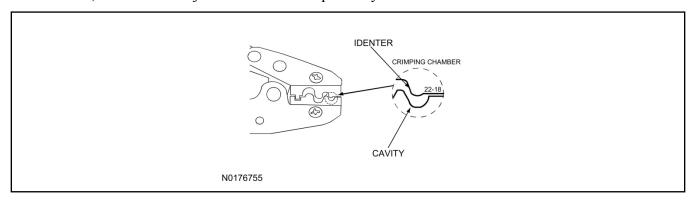
3. Center one (1) end of the butt splice on the appropriate crimping chamber. If visible, be sure to place the brazed seam of the butt splice toward the indenter. Hold the butt splice in place and squeeze the tool handles together until the ratchet engages sufficiently to hold the butt splice in position (typically one (1) or two (2) clicks). DO NOT deform the butt splice. Insert stripped wire into the butt splice, making sure the insulation on wire does not enter the butt splice.
