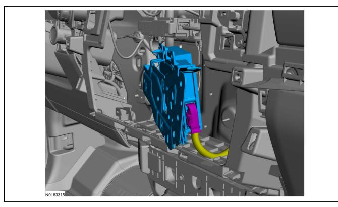
**NOTE:**Navigator, The enhanced central gateway (ECG) is located on the Driver Side C-Pillar. For additional
