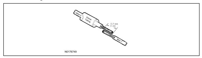
6. Overlap heat shrink tubing on both wires.
