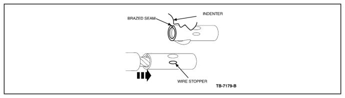
4. Holding the wire in place, squeeze tool handles together until ratchet releases. Allow tool handles to open, then remove crimped butt splice.
