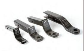
We offer square-shank **drawbars** for hitches with 1-1/4", 2" and 2-1/2" square receivers. Coated with a durable black powdercoat finish, kits include the drawbar, pin and retaining clip. A Pintle Mount is also available for 2-1/2" receivers.
