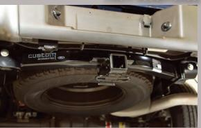
**Hitch assemblies** that allow towing capacities up to 20,000 lbs. are available for your Ford truck. Each was designed for your specific vehicle and bolts directly to the frame with no cutting or welding required. A corrosion-resistant black finish is used to give the hitch a custom look.
