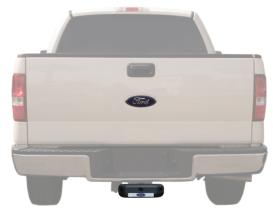
The system activates when the vehicle is engaged into reverse gear and HitchScan® starts to silently scan behind the vehicle.
