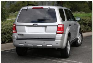
The Rear Sensing System provides up to 7 feet of coverage behind the vehicle. When the vehicle is engaged in reverse gear, the ultrasonic sensors start silently scanning behind the vehicle.
