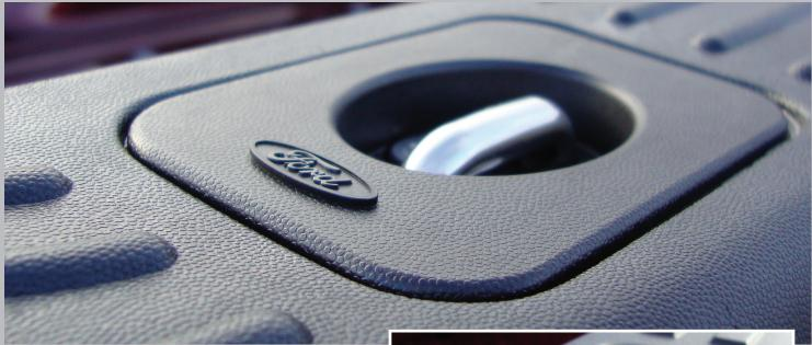
BullRing® retractable tie-downs provide you with excellent anchor points to help you secure that bulky load. BullRing® retractable tie-downs are rated with a capacity of up to 1,000 pounds. With the load properly secured with the correct tie-down straps, you can hit the road with the confidence your load will remain in place until you want it to move.
