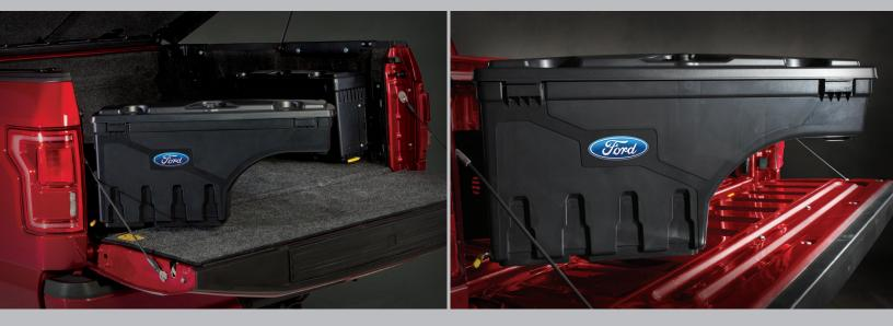
Pivot Storage Box fits in the area between the wheel well and the back of the bed and provides a rugged, weather-resistant storage compartment for tools or other gear normally just tossed into the truck bed.
