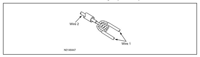
4. Evenly position heat shrink tubing over wire repair.
