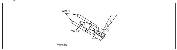
3. Bend Wire #1 back over the twisted wires for sealing. Inspect solder joint bond.
