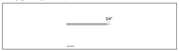
2. On the vehicle wire to be spliced into, carefully spread ½" (12.7mm) of insulation from the wire with the wire stripping tool. Inspect the wire for broken strands. If broken strands are present see "Wiring Repair Job Aid" for repair procedures.
