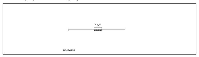
3. Tightly wrap the new wire around the vehicle wire. Solder the wire together.
