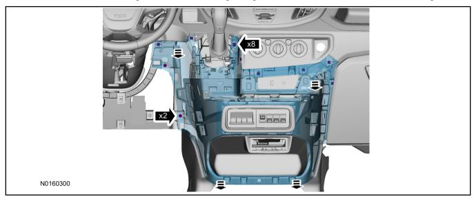
16. Remove the steering column opening reinforcement panel.
