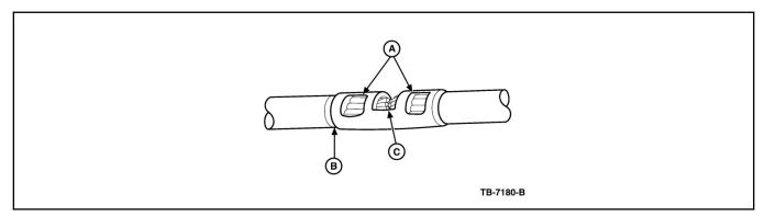
Overlap heat shrink tubing on both wires.
