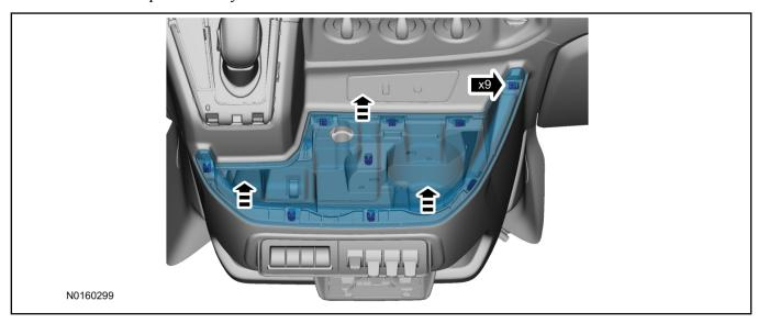
15. Remove the two screws, pull to release the eight clips and remove the center console finish panel.
