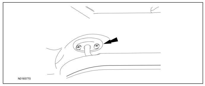
20. Remove the LH sun visor retaining clip screw and retaining clip.
