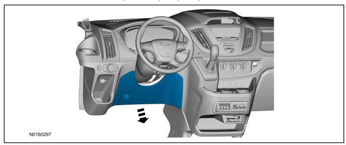
10. Remove the LH side cup holder from the instrument panel.
