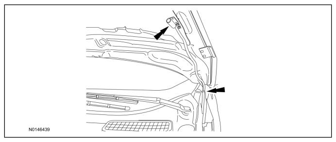
43. Connect the hood switch ground wire to a suitable location.
