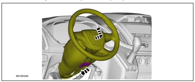
18. Position steering wheel and disengage upper shroud from lower shroud.
