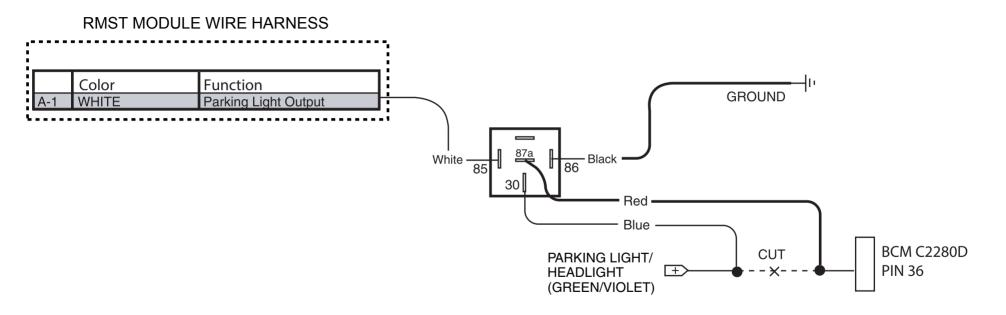
NOTE: REMOVE THE YELLOW WIRE AND TERMINAL FROM THE RELAY SOCKET
