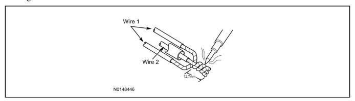
16. Bend Wire #1 back over the twisted wires for sealing. Inspect solder joint bond.
