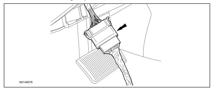
9. Connect T-harness to the back of the gateway module.
