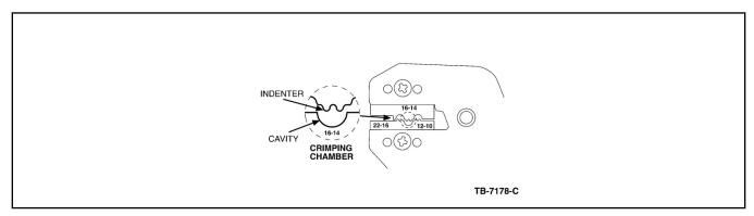
9. Center one (1) end of the butt splice on the appropriate crimping chamber. If visible, be sure to place the brazed seam of the butt splice toward the indenter. Hold the butt splice in place and squeeze the tool handles together until the ratchet engages sufficiently to hold the butt splice in position (typically one (1) or two (2) clicks). DO NOT deform the butt splice. Insert stripped wire into the butt splice, making sure the insulation on wire does not enter the butt splice.
