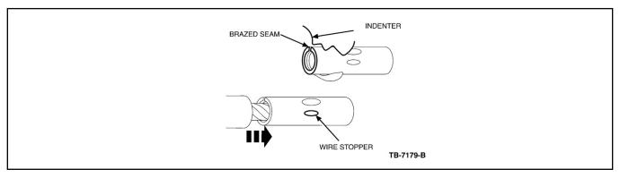
10. Holding the wire in place, squeeze tool handles together until ratchet releases. Allow tool handles to open, then remove crimped butt splice.
