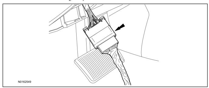
8. Connect T-harness to the back of the gateway module.
