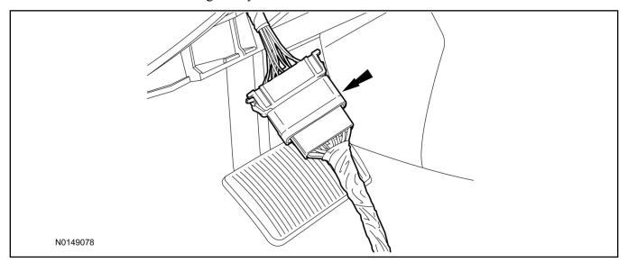
7. Connect the T-harness to the back of the gateway module.
