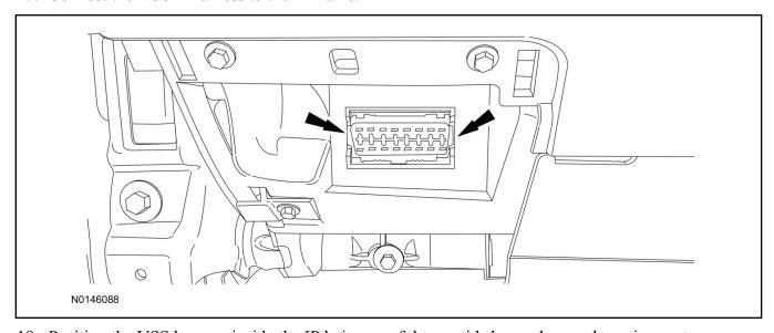
18. Position the VSS harness inside the IP being careful to avoid sharp edges and moving parts.
