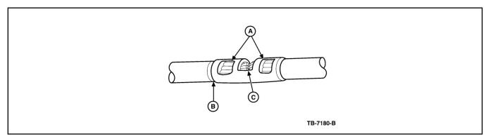
Overlap heat shrink tubing on both wires.
