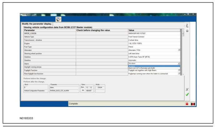
104.Identify the "Remote Start" parameter and change the value from "Less Remote Starter" to "Remote Starter".
