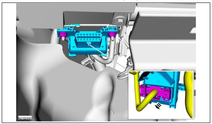
7. Connect the T-harness to the gateway module electrical connector.
