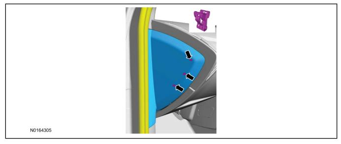
59. Clean the antenna mounting surface using an alcohol base solution and a clean cloth.
