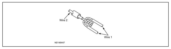
17. Evenly position heat shrink tubing over wire repair.
