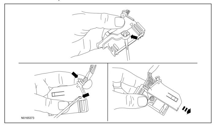
53. If equipped, remove the pin plug from BCM connector C2280A Pin 15.
