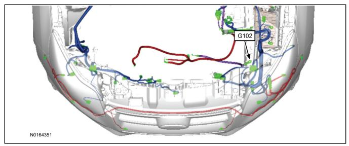
50. Route the hood latch wire harness into the vehicle through the bulkhead grommet.
