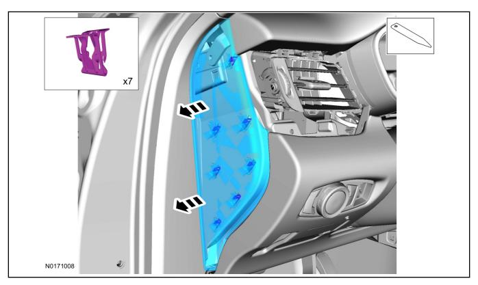
32. Position aside the LH weatherstrip and remove the upper cowl side trim panel.
