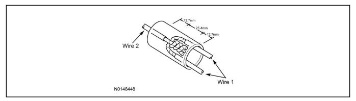
Durability of a heat shrink tubing splice is dependent on the hot melt that will appear from both ends of the tube.
