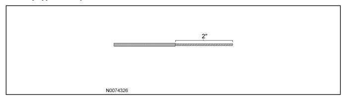
2. On the vehicle wire to be spliced into, strip one inch of insulation from the wire.
