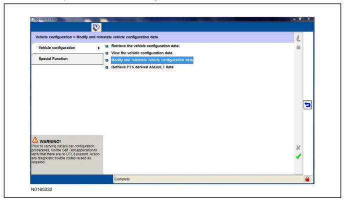
33. Identify the "Alarm" parameter and change the value from "No alarm" to "Alarm not CAT 1 (Perimeter anti-theft)".
