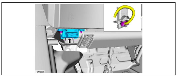
8. Connect the T-harness to the gateway module electrical connector.
