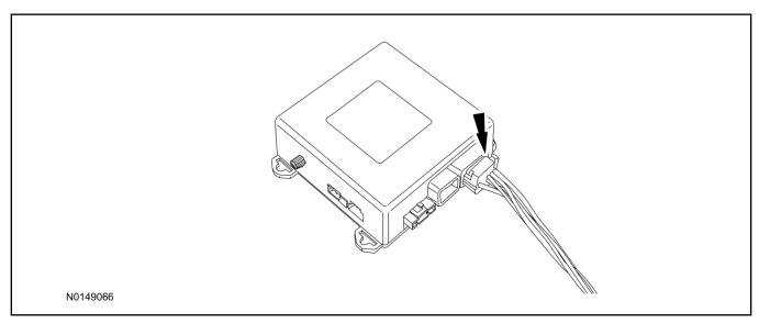
11. Install the gateway module. For additional information, refer to WSM Section 418-00.
