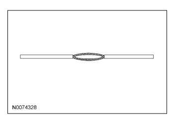
4. Insert the new wire between the parted strands. If more than one wire is being spliced, wrap them in opposite directions.
