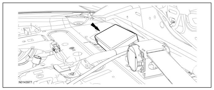
11. Connect the female end of the 8-pin T-harness to the TPM module.
