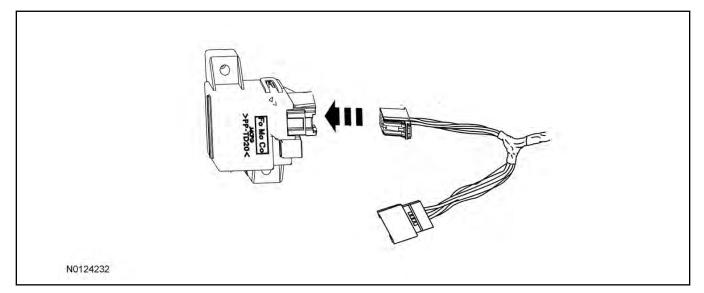
12. Connect the male end of the 8-pin T-harness to the vehicle's existing TPM module harness.
