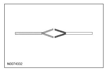
2. Place the wires next to each other and twist the upper and lower strands together as shown.
