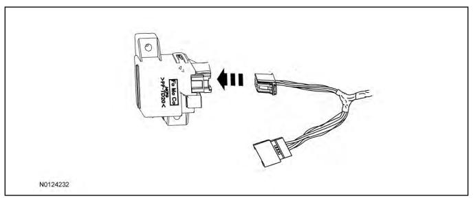
9. Connect the male end of the 8-pin T-harness to the vehicle's existing TPM module harness.
