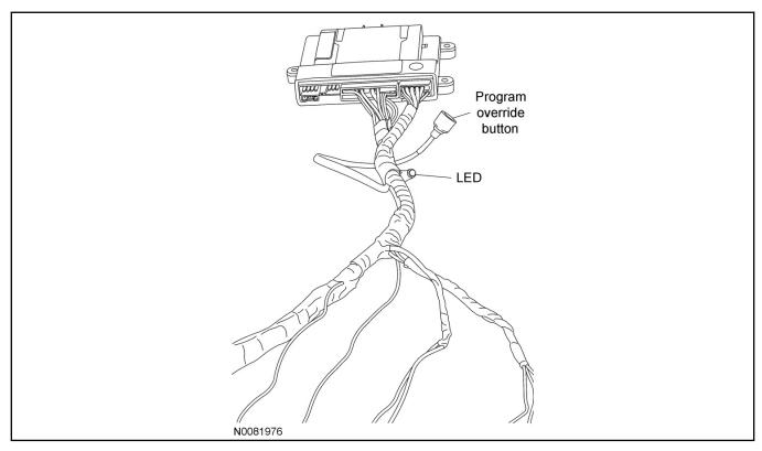
8. Tape the harness sections together, making sure to cover all of the unused wires.
