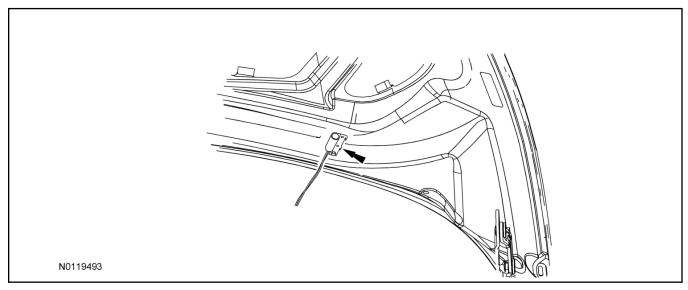
56. Connect the hood switch ground wire to a suitable location on the bulkhead.
