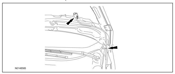
44. Connect the hood switch ground wire to a suitable location.
