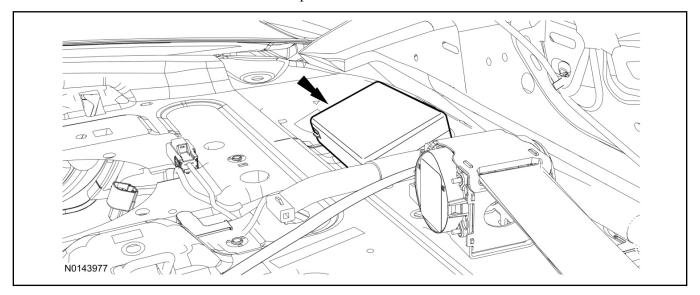
8. Connect the female end of the 8-pin T-harness to the TPM module.
