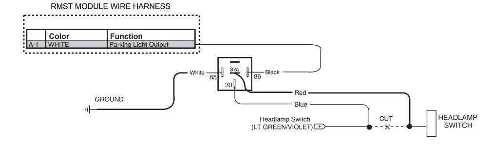
NOTE: REMOVE THE YELLOW WIRE AND TERMINAL FROM THE RELAY SOCKET
