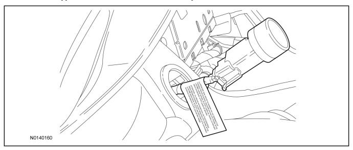
17. Install the start/stop switch. For additional Information, refer to WSM, Section 211-05.
