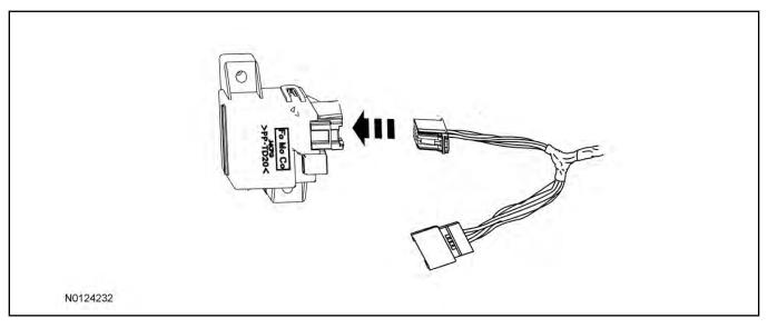
13. Connect the male end of the 8-pin T-harness to the vehicle's existing TPM module harness.
