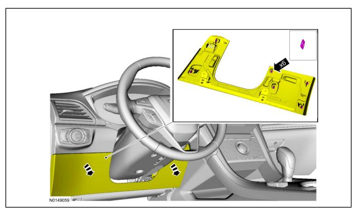
5. Position aside the LH weather strip and remove the LH Instrument Panel (IP) side trim panel.
