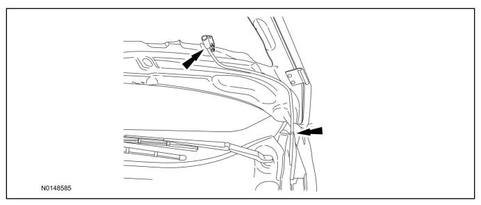
53. Connect the hood switch ground wire to a suitable location.
