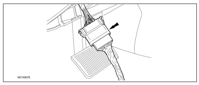
9. Connect RMST T-harness to the back of the gateway module.
