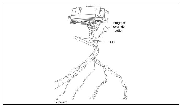
8. Tape the harness sections together, making sure to cover all of the unused wires.
