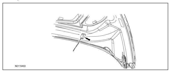
42. Connect hood switch ground wire to a suitable location on the bulkhead.
