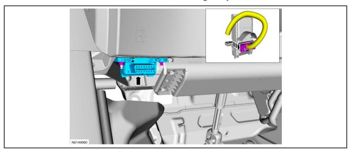
8. Connect the RMST T-harness to the gateway module electrical connector.
