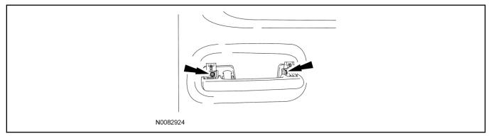
38. Pull downward on the overhead console to release the retainer clips.
