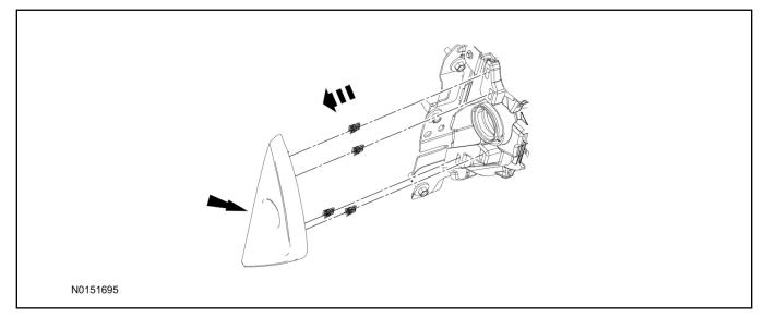
29. Clean the antenna mounting surface using an alcohol base solution and a clean cloth.
