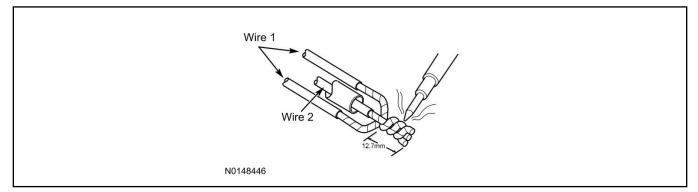
16. Bend Wire #1 back over the twisted wires for sealing. Inspect solder joint bond.
