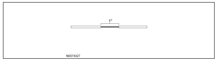
3. On the vehicle wire to be spliced into, separate the strands to allow the new wire to be placed.
