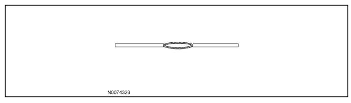
4. Insert the new wire between the parted strands. If more than one wire is being spliced, wrap them in opposite directions.
