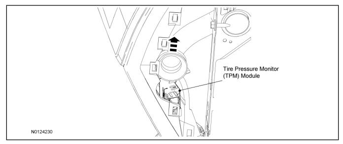
41. Position the A/C duct to access the TPM module electrical connectors.
