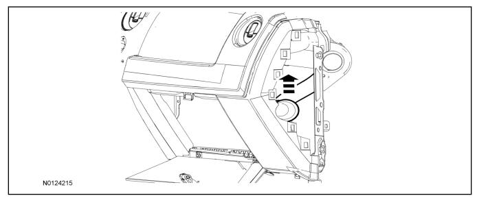
42. Connect the antenna jumper wire to the TPM module.
