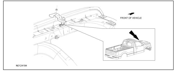
36. Connect the electrical connector to the hood switch.
