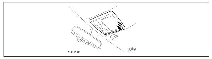
39. Disconnect the overhead console electrical connector(s) and remove the overhead console.
