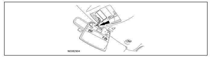
40. Remove the headliner push pin retainer.
