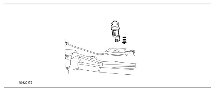
35. Connect the electrical connector to the hood switch.
