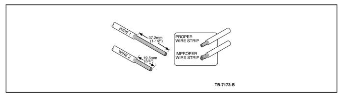
Use rosin core mildly activated (RMS) solder. do not use acid core solder for wire repair.
