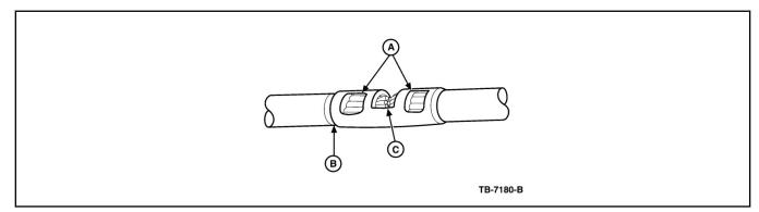
Overlap heat shrink tubing on both wires.
