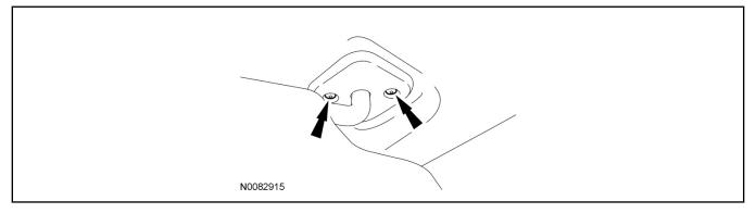
35. Remove the RH sun visor clip retainer screws and remove the sun visor clip.
