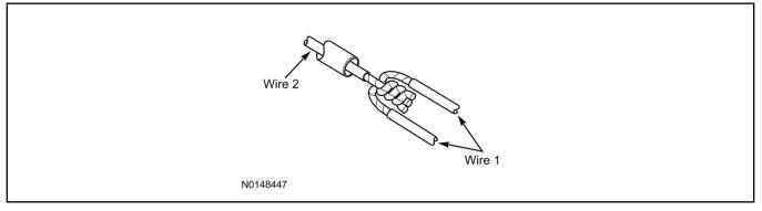
17. Evenly position heat shrink tubing over wire repair.
