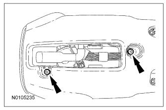
17. Remove the lower steering column shroud.
