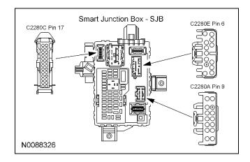
33. **NOTE:** A DVOM connected to the correct wire will show 0V, then show 12V while depressing the brake pedal.
