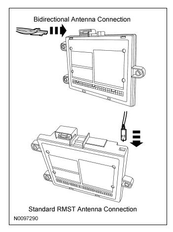
23. Connect the SECURILOCK interface module to the RMST control module.
