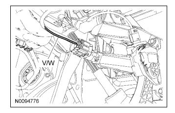
34. **NOTE:** A DVOM connected to the correct wire will show 12V with the vehicle door(s) open and the dome light on, then show 0V with the vehicle door(s) closed and the dome light off.
