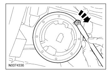
17. *NOTICE:* Do not damage the transceiver ring during installation or while installing the steering column shroud.
