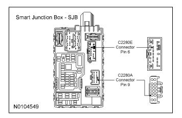
Connect the White wire from the remote start module harness to the Violet/White parking light circuit wire at the SJB C2280E Connector Pin 6.
