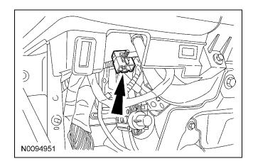
22. Connect the antenna to the RMST control module.
