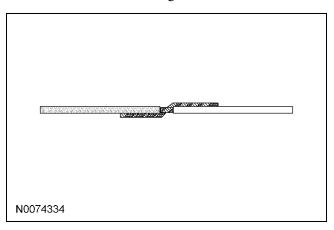
4. Wrap the connection with electrical tape so the tape covers the wires approximately two inches on either side of the connection.
