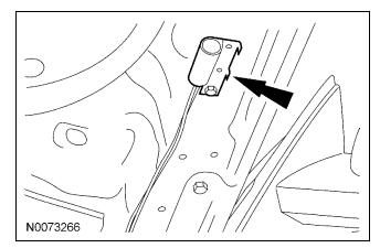
45. Connect hood switch ground wire to a suitable location on the bulkhead.
