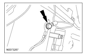
31. Disconnect the ignition switch electrical connector.
