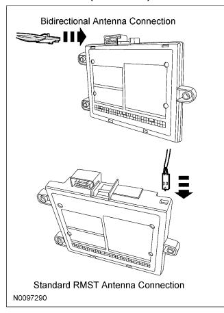
57. Connect the SECURILOCK interface module to the RMST control module.
