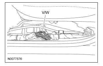
51. Connect the White wire from the control module harness to the Violet/White parking lights on circuit wire at the driver sill plate harness location.
