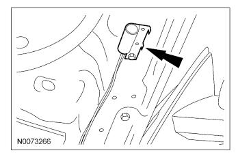
76. Connect hood switch ground wire to a suitable location on the bulkhead.
