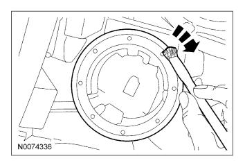
19. *NOTICE:* Do not damage the transceiver ring during installation or while installing the steering column shrouds.
