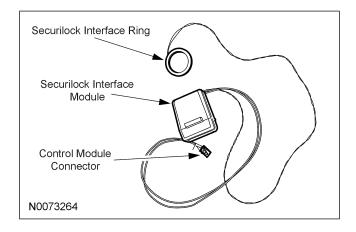
18. Following the directions on the supplied tube of adhesive primer, apply a thin coating around the transceiver antenna coil and allow to dry for approximately 5 minutes.
