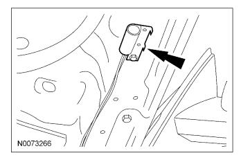
65. Connect hood switch ground wire to a suitable location on the bulkhead.
