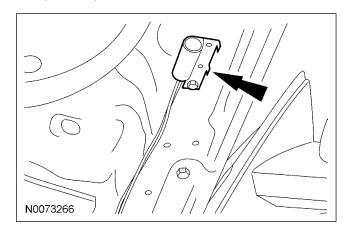
64. Connect hood switch ground wire to a suitable location on the bulkhead.
