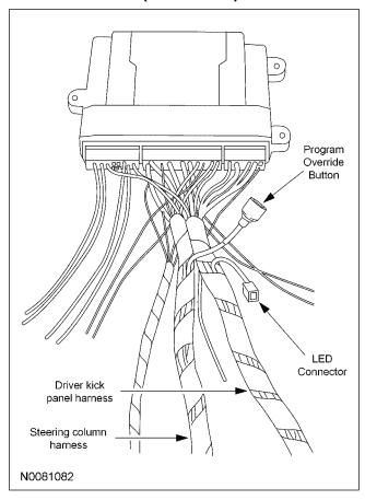
9. Tape the harness sections together, making sure to cover all of the unused wires.
