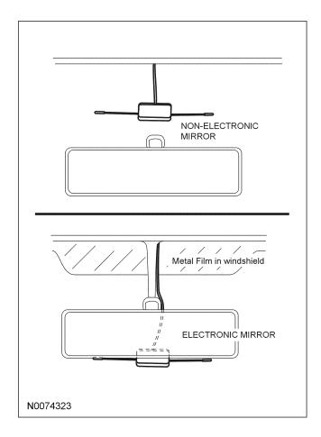
16. Route the dipole antenna cable along the headliner and down the A pillar toward the floor. The wire can be tucked behind the headliner without removing or loosening any of the trim panels.
