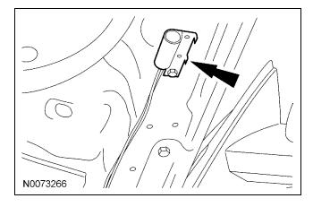
61. Connect hood switch ground wire to a suitable location on the bulkhead.
