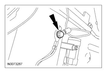
24. **NOTE:** A DVOM connected to the correct wire will show 0V, then show 12V when the Ignition Switch is in the RUN and START positions.
