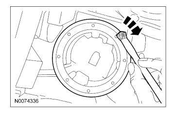
22. *NOTICE:* Do not damage the transceiver ring during installation or while installing the steering column shrouds.
