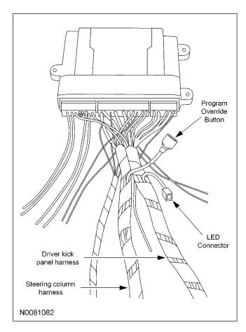
10. Tape the harness sections together, making sure to cover all of the unused wires.
