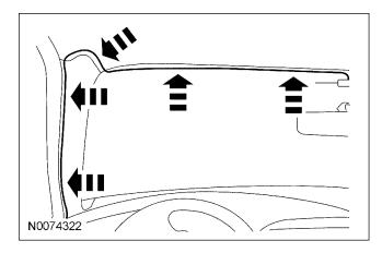
21. Route the ring of the SECURILOCK interface antenna lead up along the steering column to the PATS transceiver location.
