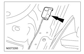
64. Connect hood switch ground wire to a suitable location on the bulkhead.
