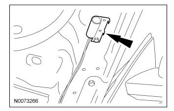
63. Connect hood switch ground wire to a suitable location on the bulkhead.
