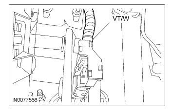
35. Connect the Brown wire from the control module harness B-7 to the Violet/White brake switch circuit wire at the brake switch.
