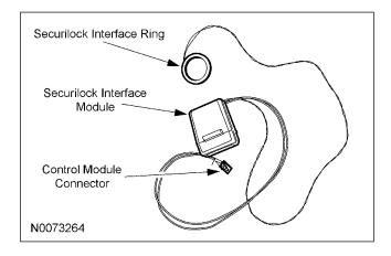
18. Following the directions on the supplied tube of adhesive primer, apply a thin coating around the transceiver antenna coil and allow to dry for approximately 5 minutes.
