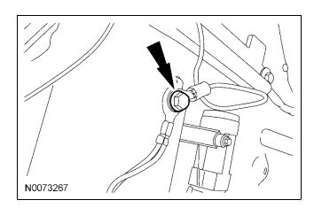
23. **NOTE:** A DVOM connected to the correct wire will show 0V, then show 12V when the ignition switch is in the RUN/START position.
