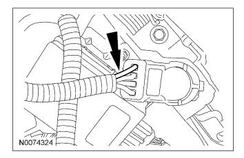
37. Connect the Brown wire from the control module harness to the Violet/White brake switch circuit wire at the driver kick panel harness. 38. **NOTE:** A DVOM connected to the correct wire will show 12V, when the Headlight Switch is in the park lamp position, then show 0V when the Headlight Switch is OFF.
