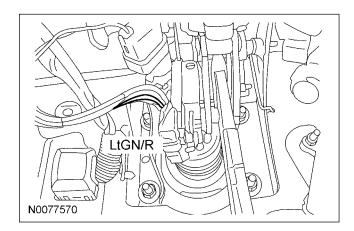
50. Connect the Brown wire from the control module harness to the Light Green/Red brake switch circuit wire at the brake switch.
