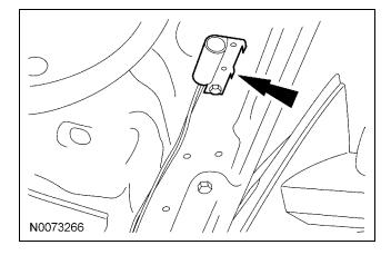
69. Connect hood switch ground wire to a suitable location on the bulkhead.
