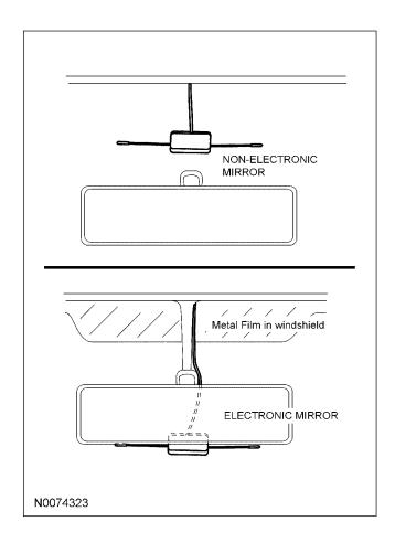
17. Route the dipole antenna cable along the headliner and down the A pillar toward the floor. The wire can be tucked behind the headliner without removing or loosening any of the trim panels.
