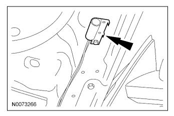
63. Connect hood switch ground wire to a suitable location on the bulkhead.
