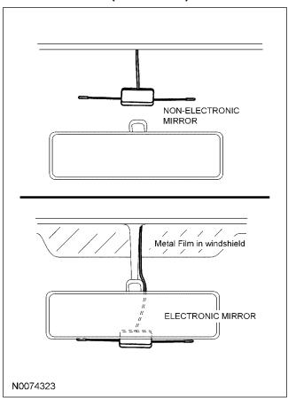
15. Route the dipole antenna cable along the headliner and down the A pillar toward the floor. The wire can be tucked behind the headliner without removing or loosening any of the trim panels.
