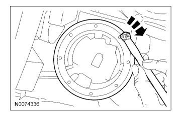
18. *NOTICE:* Do not damage the transceiver ring during installation or while installing the steering column shrouds.
