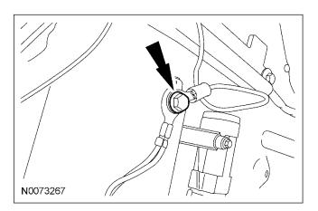
31. **NOTE:** A DVOM connected to the correct wire will show 0V, then show 12V when the Ignition Switch is in the RUN and START positions.
