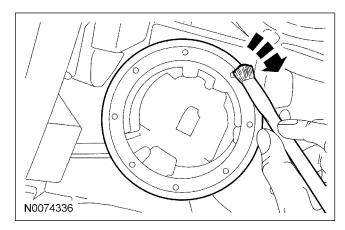
21. *NOTICE:* Do not damage the transceiver ring during installation or while installing the steering column shrouds.
