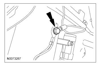
23. **NOTE:** A DVOM connected to the correct wire will show 0V when the ignition switch is in the OFF position, then show 12V with the ignition switch in the RUN/START position.
