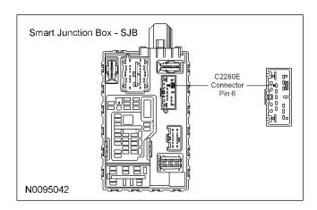
55. Connect the White wire from the control module harness to the Violet/White parking light circuit wire at the SJB C2280E Connector Pin 6.
