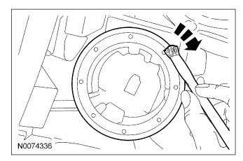
26. *NOTICE:* Do not damage the transceiver ring during installation or while installing the steering column shroud.
