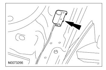
68. Connect hood switch ground wire to a suitable location on the bulkhead.
