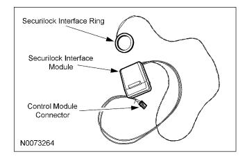
25. Following the directions on the supplied tube of adhesive primer, apply a thin coating around the transceiver antenna coil and allow to dry for approximately 5 minutes.
