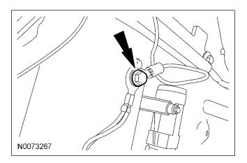
31. **NOTE:** A DVOM connected to the correct wire will show 12V, then show 0V when the horn button is held.
