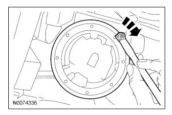
20. *NOTICE:* Do not damage the transceiver ring during installation or while installing the steering column shroud.
