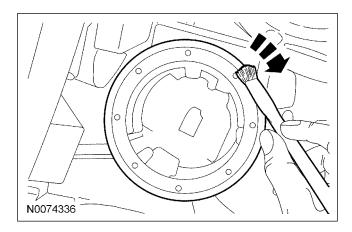
22. *NOTICE:* Do not damage the transceiver ring during installation or while installing the steering column shrouds.
