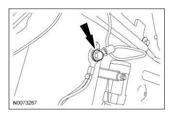
25. Disconnect the ignition switch electrical connector.
