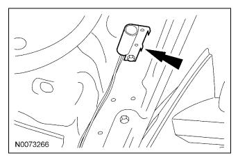
39. Connect hood switch ground wire to a suitable location on the bulkhead.
