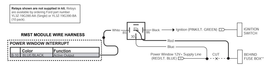
\*\*Fuse box must be removed by uncliping and sliding back to access the RED/LT. BLUE wire located behind fuse #42 on the right side.
