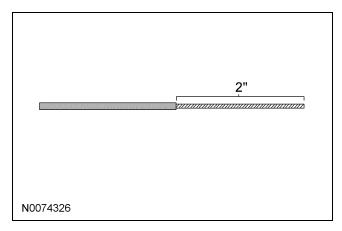
2. On the vehicle wire to be spliced into, strip one inch of insulation form the wire.
