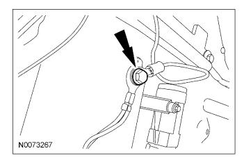
29. **NOTE:** A DVOM connected to the correct wire will show 12V, then show 0V when the horn button is held.
