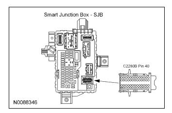
35. **NOTE:** A DVOM connected to the correct wire will show 12V with the vehicle door(s) open and the dome light on, then show 0V with the vehicle door(s) closed and the dome light off.
