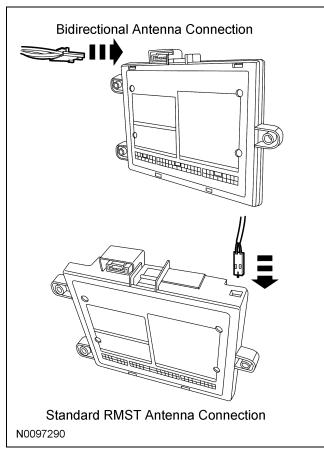
45. Connect the SECURILOCK interface module to the RMST control module.
