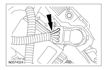
38. Connect the Brown wire from the remote start module harness to the Violet/White brake switch circuit wire at the brake switch.
