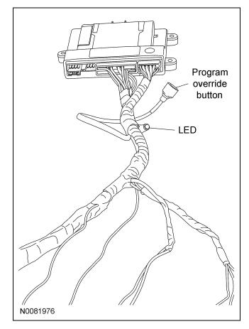
8. Tape the harness sections together, making sure to cover all of the unused wires.
