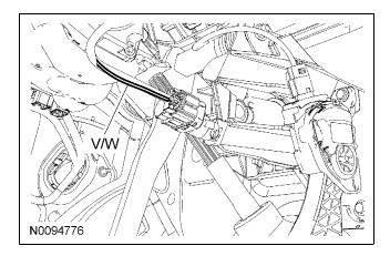
34. **NOTE:** A DVOM connected to the correct wire will show 12V with the vehicle door(s) open and the dome light on, then show 0V with the vehicle door(s) closed and the dome light off.
