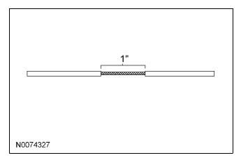
3. On the vehicle wire to be spliced into, separate the strands to allow the new wire to be placed between the parted strands of wire.
