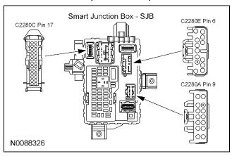
33. **NOTE:** A DVOM connected to the correct wire will show 0V, then show 12V while depressing the brake pedal.
