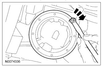
16. *NOTICE:* Do not damage the transceiver ring during installation or while installing the steering column shroud.
