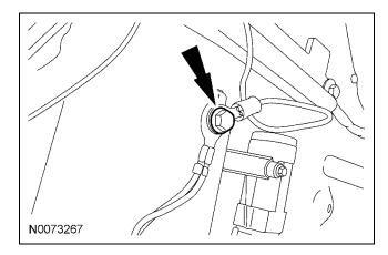
28. **NOTE:** A DVOM connected to the correct wire will show 12V, then show 0V when the horn button is held.
