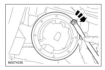
20. *NOTICE:* Do not damage the transceiver ring during installation or while installing the steering column shrouds.
