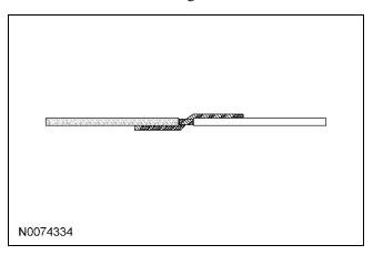
4. Wrap the connection with electrical tape so the tape covers the wires approximately two inches on either side of the connection.
