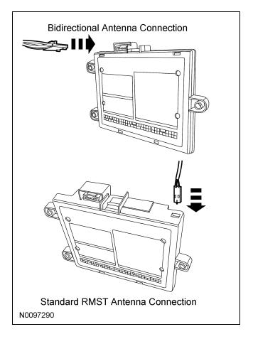
43. Connect the SECURILOCK interface module to the RMST control module.
