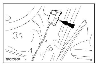
41. Connect hood switch ground wire to a suitable location on the bulkhead.
