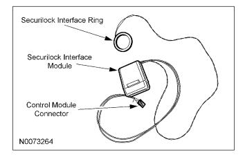
22. Following the directions on the supplied tube of adhesive primer, apply a thin coating around the transceiver antenna coil and allow to dry for approximately 5 minutes.
