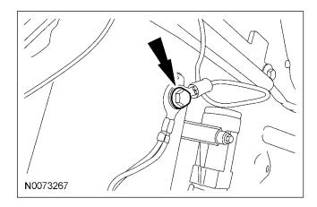
32. **NOTE:** A DVOM connected to the correct wire will show 12V, then show 0V when the horn button is held.
