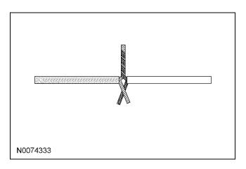
**NOTE:** Use Rosin Core Mildly-Activated (RMA) Solder. Do not use Acid Core Solder.
