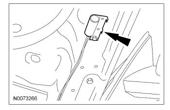
39. Connect hood switch ground wire to a suitable location on the bulkhead.
