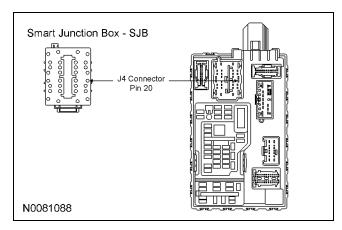
38. Connect the White wire from the remote start module harness to the Violet/White parking light circuit wire at the SJB J4 Connector Pin 20.
