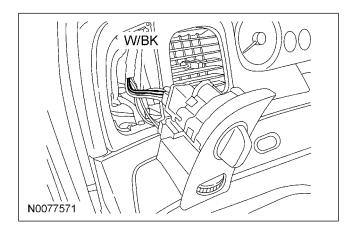
31. **NOTE:** A DVOM connected to the correct wire will show 0V, then show 12V when the door lock switch is pressed.
