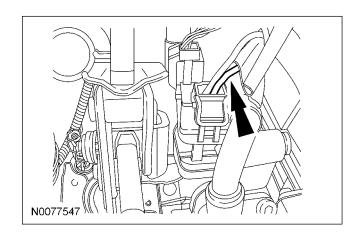
39. **NOTE:** A DVOM connected to the correct wire will show 12V with the vehicle door(s) open and the dome light on, then show 0V with the vehicle door(s) closed and the dome light off.
