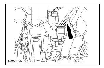
35. **NOTE:** A DVOM connected to the correct wire will show 12V, when the headlight switch is ON, then show 0V when the headlight switch is OFF.
