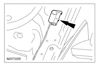
46. Connect hood switch ground wire to a suitable location on the bulkhead.
