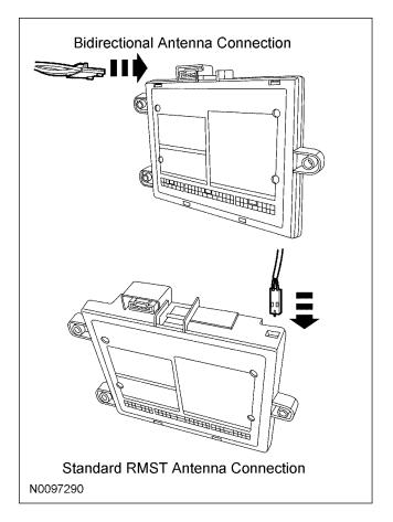
50. Connect the SECURILOCK interface module to the RMST control module.
