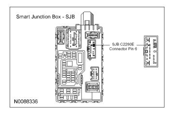
37. **NOTE:** A DVOM connected to the correct wire will show 0V, then show 12V while depressing the brake pedal.
