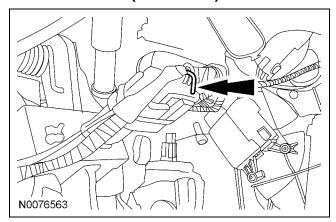
33. **NOTE:** A DVOM connected to the correct wire will show 12V with the vehicle door(s) open and the dome light ON, then show 0V with the vehicle door(s) closed and the dome light OFF.
