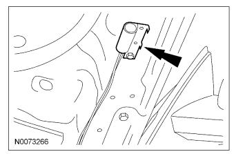
43. Connect hood switch ground wire to a suitable location on the bulkhead.
