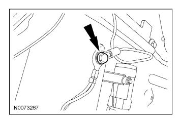
25. Disconnect the ignition switch electrical connector.
