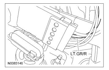
35. **NOTE:** A DVOM connected to the correct wire will show 12V with the vehicle door(s) open and the dome light ON, then show 0V with the vehicle door(s) closed and the dome light OFF.
