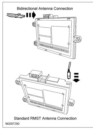
44. Connect the SECURILOCK interface module to the RMST control module.
