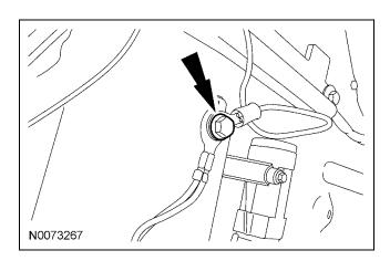
25. Disconnect the ignition switch electrical connector.
