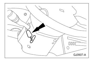
**NOTE:** Release the upper steering column shroud by pressing the sides inward.
