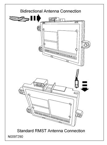
47. Connect the SECURILOCK interface module to the RMST control module.
