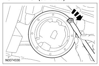
27. *NOTICE:* Do not damage the transceiver ring during installation or while installing the steering column shroud.
