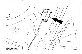
69. Connect hood switch ground wire to a suitable location on the bulkhead.
