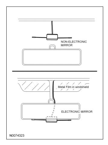
29. Route the dipole antenna cable along the headliner and down the A pillar toward the floor. The wire can be tucked behind the headliner without removing or loosening any of the trim panels.
