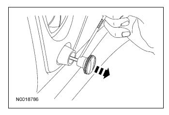
19. Remove the headlamp switch bezel by turning it counterclockwise.
