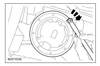
32. *NOTICE:* Do not damage the transceiver ring during installation or while installing the steering column shroud.
