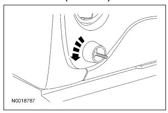
20. Remove the (2) instrument cluster finish panel screws.
