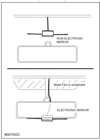
14. Route the dipole antenna cable along the headliner and down the A pillar toward the floor. The wire can be tucked behind the headliner without removing or loosening any of the trim panels.
