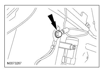
38. **NOTE:** A DVOM connected to the correct wire will show 0V, then show 12V when the Ignition Switch is in the RUN and START positions.
