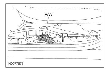
51. Connect the White wire from the control module harness to the Violet/White parking lights on circuit wire at the driver front sill plate harness location.
