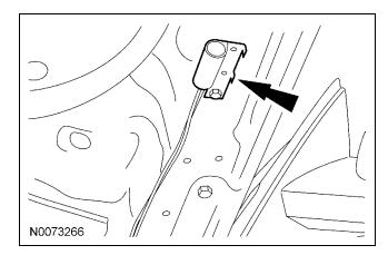
67. Connect hood switch ground wire to a suitable location on the bulkhead.
