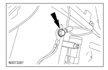
26. **NOTE:** A DVOM connected to the correct wire will show 0V, then show 12V when the Ignition Switch is in the RUN and START positions.
