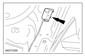
75. Connect hood switch ground wire to a suitable location on the bulkhead.
