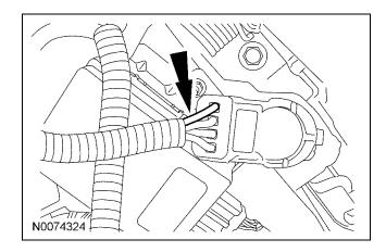
37. Connect the Brown wire from the control module harness to the Violet/White brake switch circuit wire at the driver kick panel harness.
