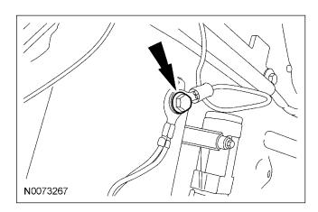
25. **NOTE:** A DVOM connected to the correct wire will show 0V, then show 12V when the ignition switch is in the RUN/START position.
