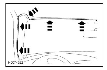
30. Route the ring of the SECURILOCK interface antenna lead up along the steering column to the PATS transceiver location.
