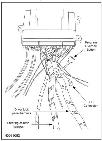
9. Tape the harness sections together, making sure to cover all of the unused wires.
