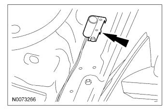
73. Connect hood switch ground wire to a suitable location on the bulkhead.
