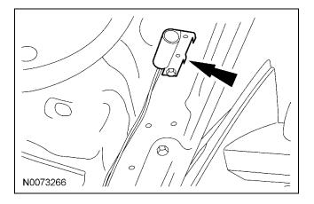
85. Connect hood switch ground wire to a suitable location on the bulkhead.
