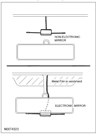
17. Route the dipole antenna cable along the headliner and down the A pillar toward the floor. The wire can be tucked behind the headliner without removing or loosening any of the trim panels.
