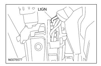
48. Connect the Brown wire from the control module harness to the Light Green brake switch circuit wire at the brake switch.
