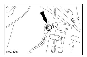
25. **NOTE:** A DVOM connected to the correct wire will show 12V with the vehicle door(s) open and the dome light on, then show 0V with the vehicle door(s) closed and the dome light off.
