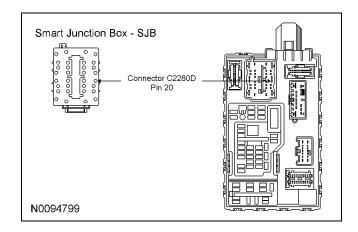
56. Connect the White wire from the control module harness to the Violet/White parking light circuit wire at the SJB Connector C2280D Pin 20.
