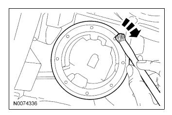
19. *NOTICE:* Do not damage the transceiver ring during installation or while installing the steering column shroud.
