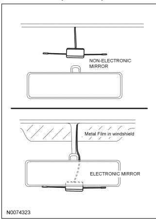
23. Route the dipole antenna cable along the headliner and down the A pillar toward the floor. The wire can be tucked behind the headliner without removing or loosening any of the trim panels.
