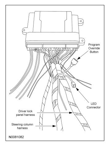
11. Tape the harness sections together, making sure to cover all of the unused wires.
