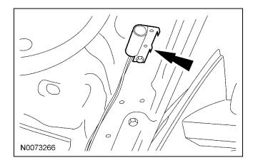
96. Connect hood switch ground wire to a suitable location on the bulkhead.
