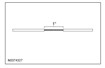
3. On the vehicle wire to be spliced into, separate the strands to allow the new wire to be placed between the parted strands of wire.
