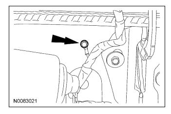
78. **NOTE:** Place the label on the radiator fan shroud or similar area.
