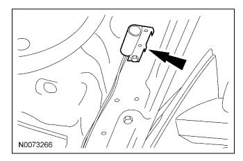
77. Connect hood switch ground wire to a suitable location on the bulkhead.
