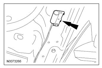
99. Connect hood switch ground wire to a suitable location on the bulkhead.
