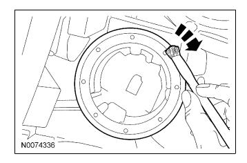
18. *NOTICE:* Do not damage the transceiver ring during installation or while installing the steering column shrouds.
