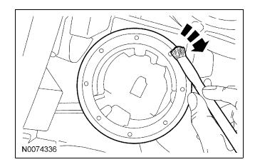
26. *NOTICE:* Do not damage the transceiver ring during installation or while installing the steering column shrouds.
