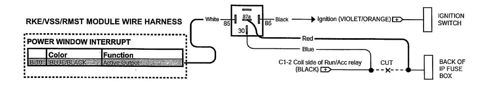
Relays shown are not supplied in kit. Relays are available by ordering Ford part number YL3Z-19G390-AA (Single) or YL3Z-19G390-BA (10 pack).
