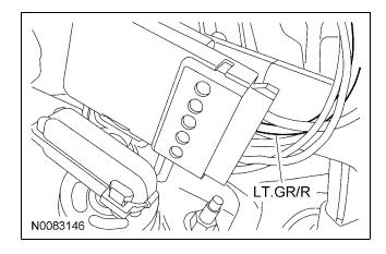
50. Connect the Brown wire from the control module harness to the Light Green/Red brake switch circuit wire at the brake switch.
