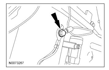
25. **NOTE:** A DVOM connected to the correct wire will show 0V, then show 12V when the Ignition Switch is in the RUN and START positions.
