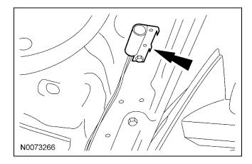
65. Connect hood switch ground wire to a suitable location on the bulkhead.
