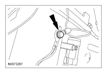
26. Disconnect the ignition switch electrical connector.
