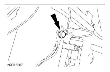
40. **NOTE:** A DVOM connected to the correct wire will show 12V, then show 0V when the horn button is held.
