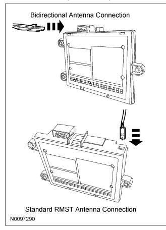
66. Connect the SECURILOCK interface module to the RMST control module.
