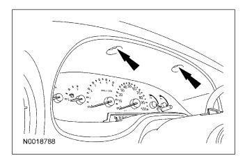
**NOTICE:** To avoid damage to the instrument cluster finish panel, pull the panel forward just enough to access the electrical connectors before completely removing the panel.
