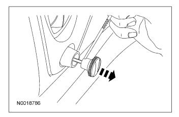
17. Remove the headlamp switch bezel by turning it counterclockwise.
