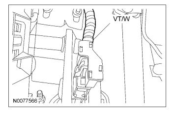
34. Connect the Brown wire from the remote start module harness to the Violet/White brake switch circuit wire at the brake switch.
