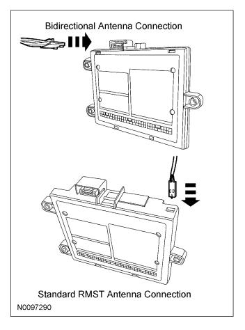
60. Connect the SECURILOCK interface module to the RMST control module.
