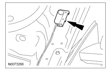
41. Connect hood switch ground wire to a suitable location on the bulkhead.
