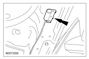
56. Connect hood switch ground wire to a suitable location on the bulkhead.
