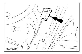
40. Connect hood switch ground wire to a suitable location on the bulkhead.
