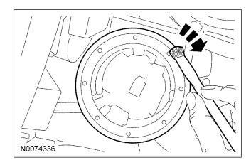
21. *NOTICE:* Do not damage the transceiver ring during installation or while installing the steering column shroud.
