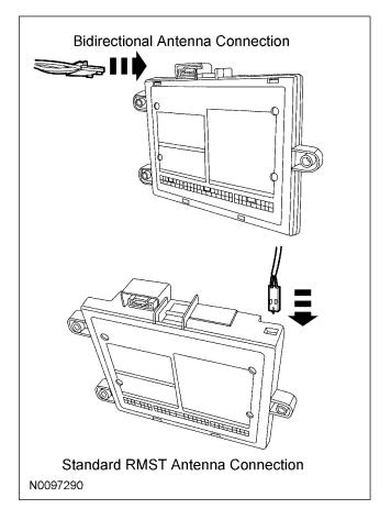
45. Connect the SECURILOCK interface module to the RMST control module.
