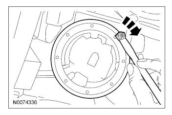
32. *NOTICE:* Do not damage the transceiver ring during installation or while installing the steering column shrouds.
