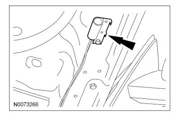
46. Connect hood switch ground wire to a suitable location on the bulkhead.
