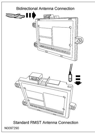
43. Connect the SECURILOCK interface module to the RMST control module.
