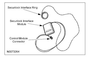
31. Following the directions on the supplied tube of adhesive primer, apply a thin coating around the transceiver antenna coil and allow to dry for approximately 5 minutes.
