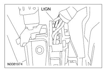
35. Connect the Brown wire from the remote start module harness to the Light Green brake switch circuit wire at the brake switch.
