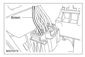
31. Connect the White wire from the remote start module harness to the Brown parking lights circuit wire at the headlight switch.
