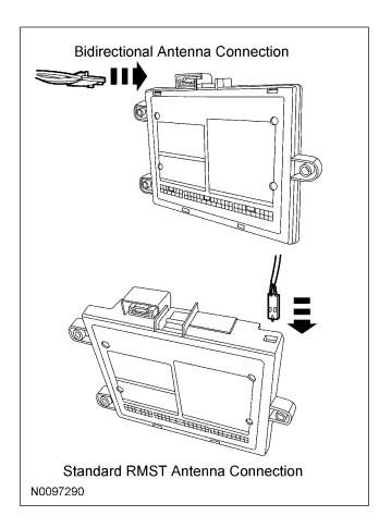
50. Connect the SECURILOCK interface module to the RMST control module.
