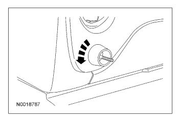
18. Remove the (2) instrument cluster finish panel screws.
