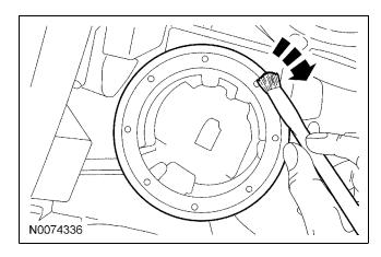
22. *NOTICE:* Do not damage the transceiver ring during installation or while installing the steering column shroud.
