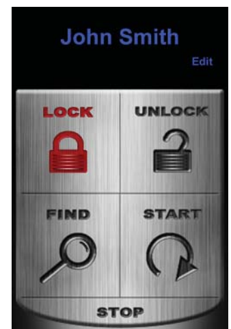
Buttons flash RED when the request could not be completed. This may be due to a cellular communication error or the state of the vehicle.
